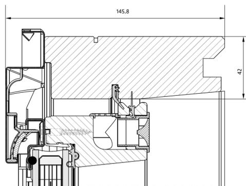
VUE DE DESSUS: OUVERTURE PAR ROTATION, DOUBLE VITRAGE
